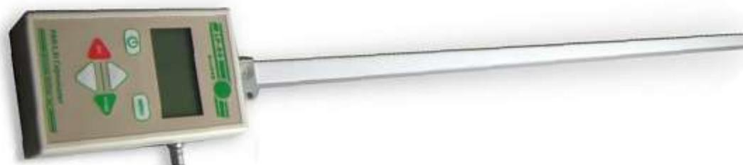
Figura 10 - Ceptômetro (LP-80 PAR/LAI, AccuPAR Decagon Devices Inc. USA).
