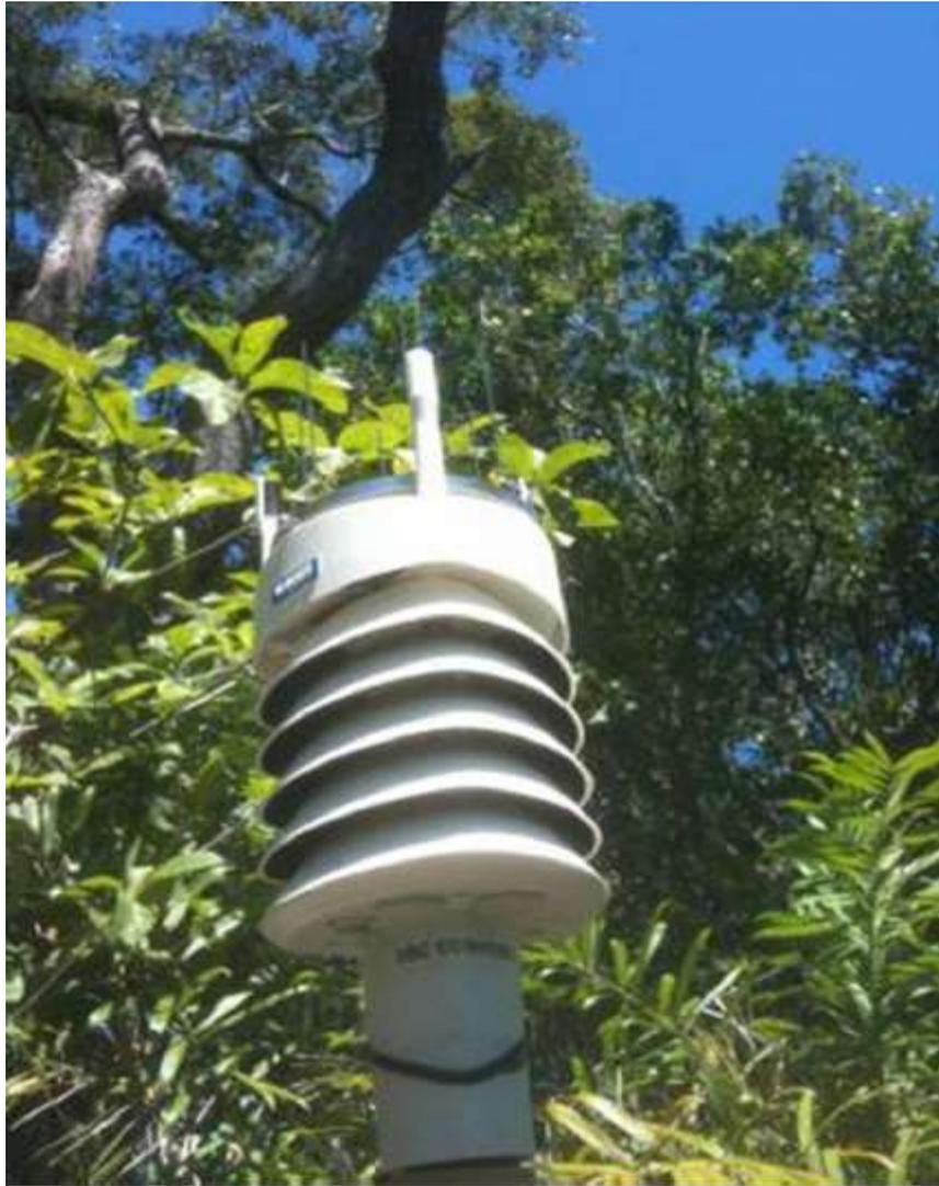
Figura 9 - Termohigrômetro (WXT520, Vaisala Inc., Helsinki, Finland).
